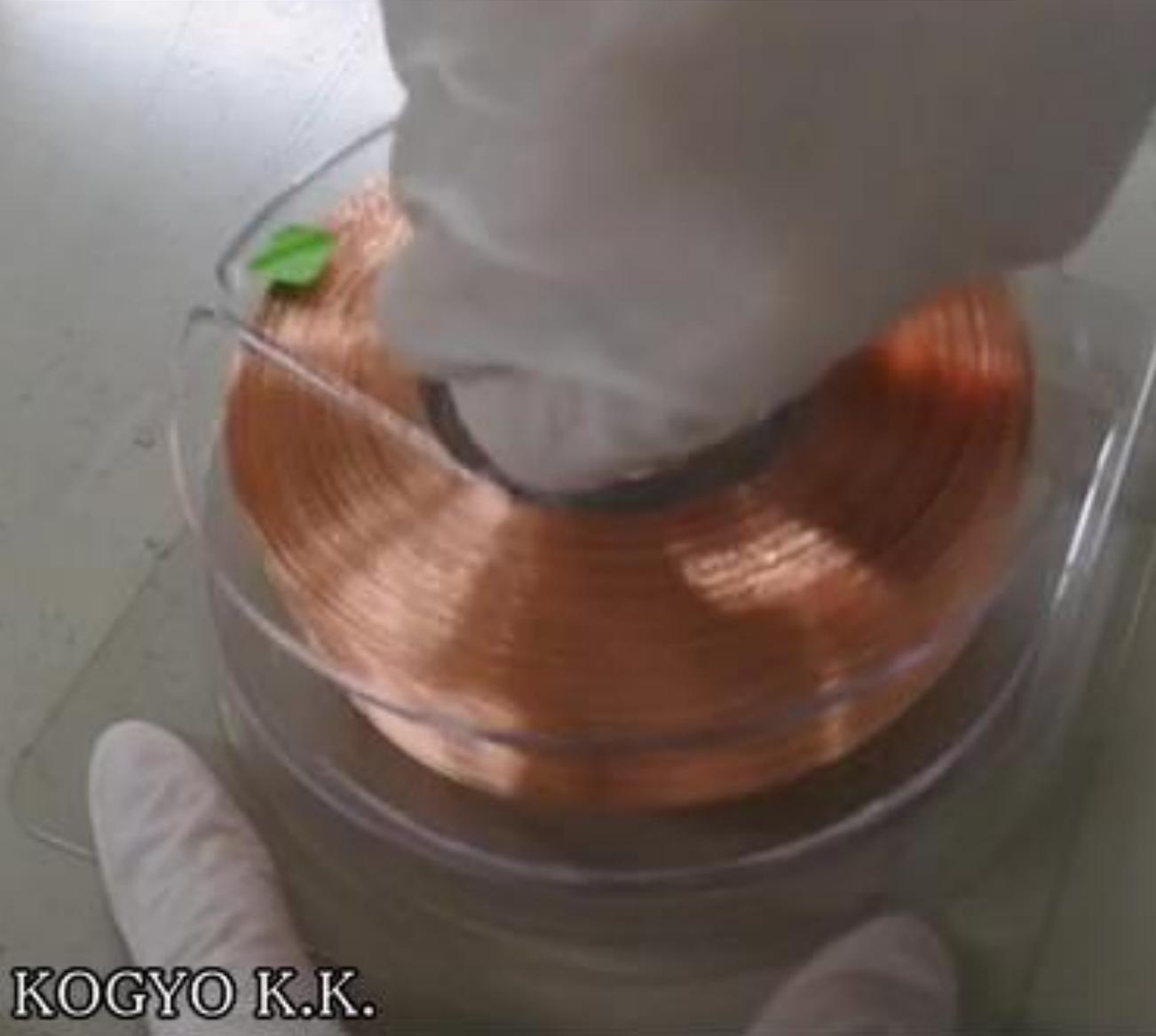
②Hold the center of the spool while pressing the bottom case and pull the spool vertically.
