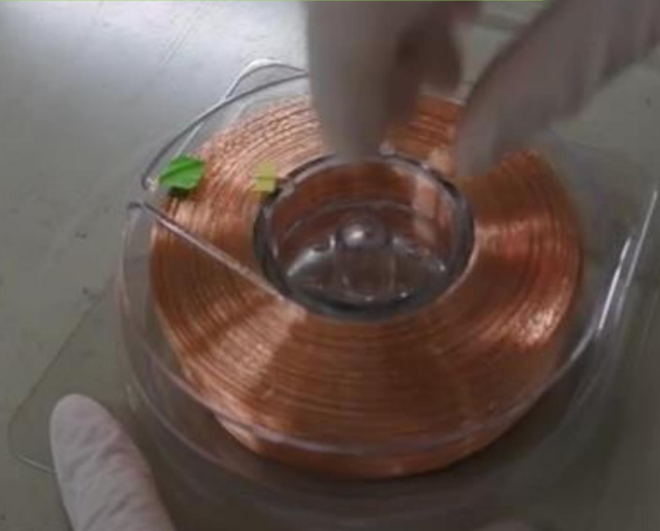
②Hold the center of the spool while pressing the bottom case and pull the spool vertically.
