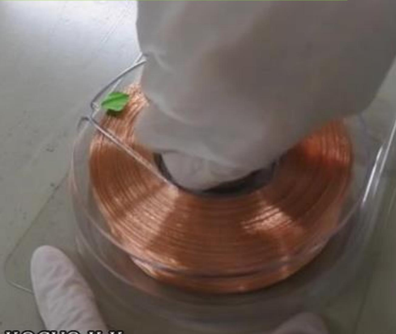
②Hold the center of the spool while pressing the bottom case and pull the spool vertically.
