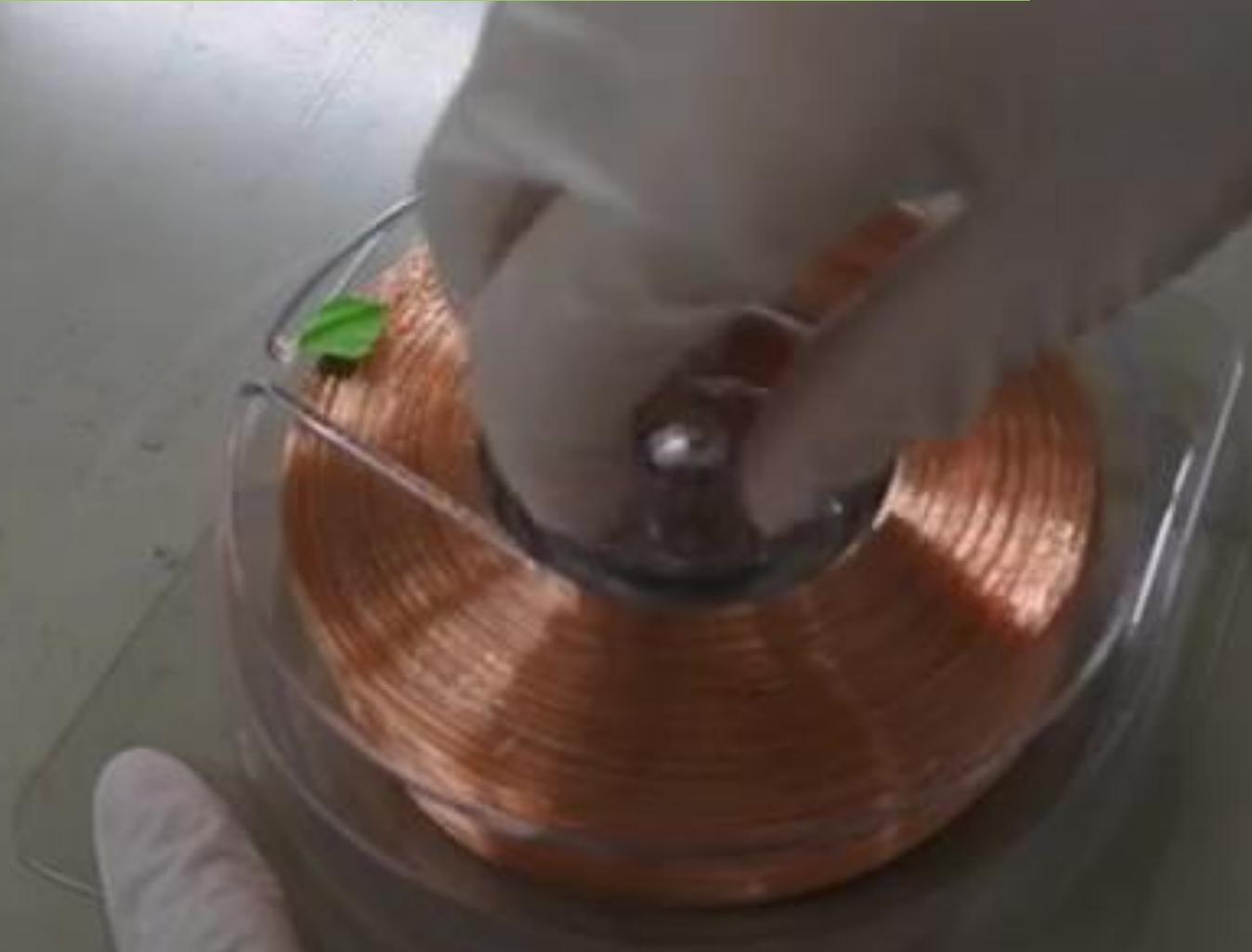
②Hold the center of the spool while pressing the bottom case and pull the spool vertically.
