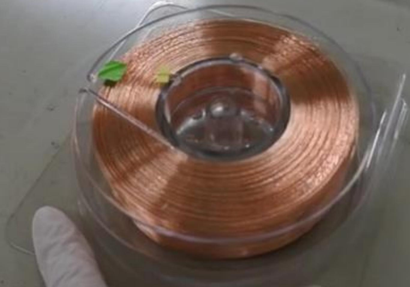
②Hold the center of the spool while pressing the bottom case and pull the spool vertically.
